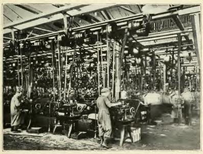
Photo from Willys-Overland, Inc. MACHINING SMALL PARTS FOR CURTISS "OX" ENGINES
